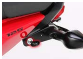
Tightens with M6 bolt. ( both right and left side)
