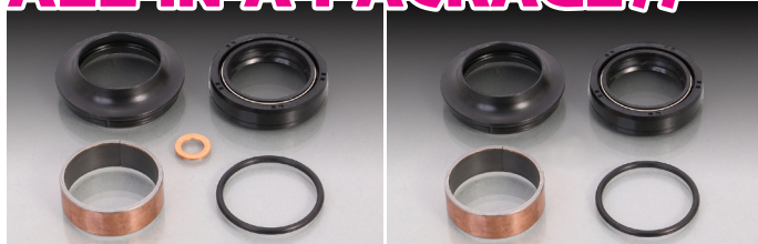
Dust seal & O-ring required for front fork maintenance and tuning.
