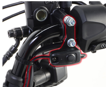
On/Off switch (push) is tightened with master cylinder.
