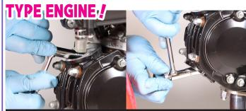
For tappet clearance adjustment and inspection for GROM / MONKEY125 type motor. Uses together with thickness gauge.
