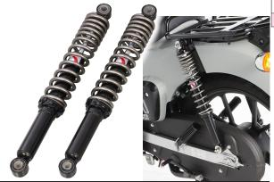
Kitaco rear shock with original oil-charged damper. Harder spring rate than stock rear shock.
