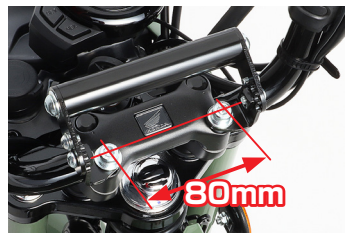
Multipurpose bar that can be changed in 5 steps (35°).
