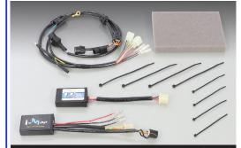
Feedback canceller set for MONKEY125 (JB02) newly released. No wiring mods required with vehicle specific coupler-on harness. Suitable map is selectable from default maps preinstalled. User original map is also editable.
