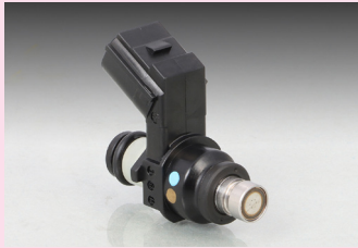
Big capacity injector (×1.3) required for big bore kit.
