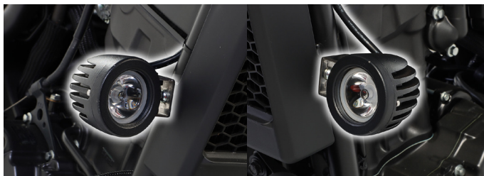
Best place for installation LED shuttle beam is mounted next to radiator.
