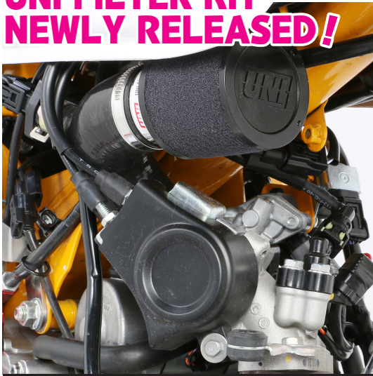
Just remove stock air cleaner box and install uni filter.
