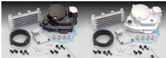
Must for high tuned engine. Prevents overheat that causes trouble of engine. Super oil cooler kit brings stable engine performance under severe circumstances to release heat as much as 400cc class oil cooler.
