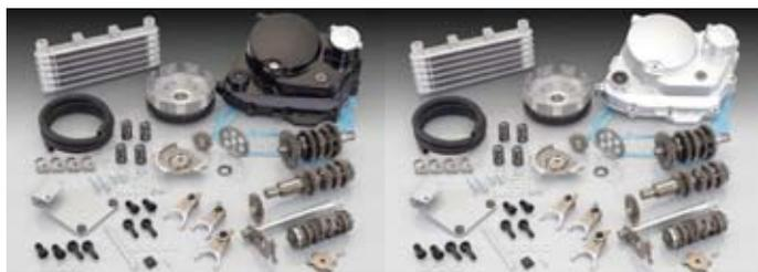
A full set that requires when using big bore kit. High quality aluminum die-cast clutch cover with oil element built-in. Comes with 6 speed transmission assy, reinforced clutch, big capacity oil cooler & big capacity oil pump. Full kit for high output for high tuned engine.
