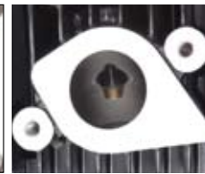
INTAKE PORT ( \phi 28) 10mm HIGH PORT
