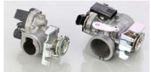
STOCK THROTTLE BODY (LEFT) & BIG THROTTLE BODY (RIGHT)
