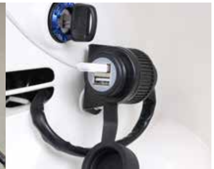
Installs the USB supply inside the right side leg shield.
