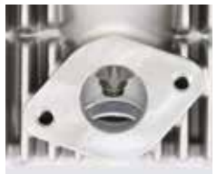
COMBUSTION CHAMBER INTAKE PORT φ 22mm EXHAUST PORT φ 18 mm
