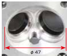
COMBUSTION CHAMBER INTAKE PORT φ 22mm EXHAUST PORT φ 18 mm
