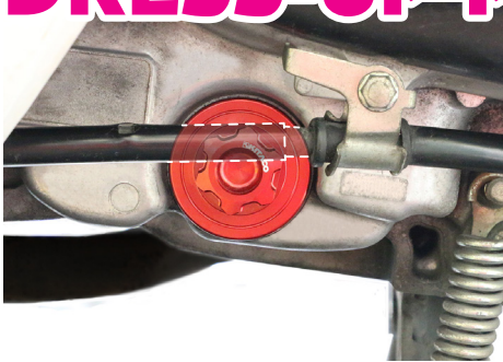
PCX (JF28) FOR OIL STRAINER CAP TORQUE 20N·m
