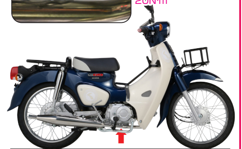
SUPER CUB 110 (JA44) FOR OIL DRAIN CAP TORQUE 20N·m
