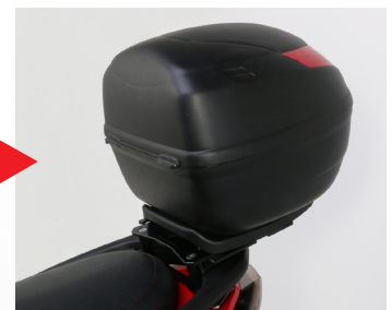
Installing rear box
