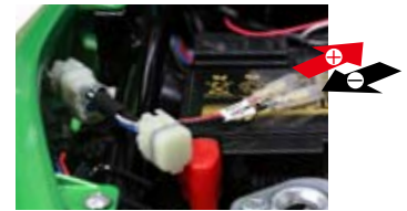
Connect power supply extract harness with removed water-proof coupler. Connect accessory such as USB battery supply with ACC⊕ GND⊖ .
