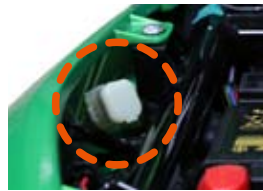
Remove 4P water-proof coupler cap
