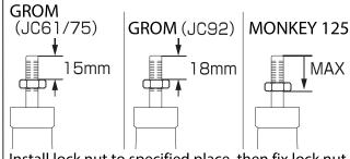
Install lock nut to specified place, then fix lock nut and tighten fork bolt.
