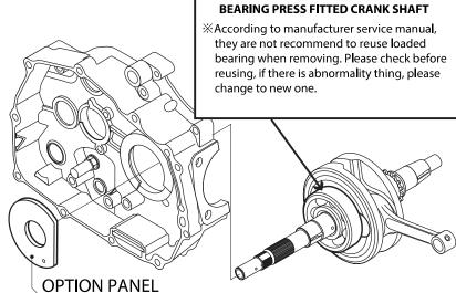
1) Place option panel and crank shaft assemble tool (sold separately) to crank case shaft, then tighten to crank shaft screw place (CW screw).
