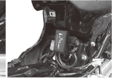
④ i-map installation point (6P coupler/terminal)
