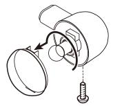
\*Hold socket and rotate flash lamp lens anticlockwise to remove.
